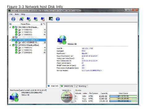
In the bottom panel, an overall status indicator shows the state of the selected network host hard disk. As well, volume details of the selected hard disk are displayed.
